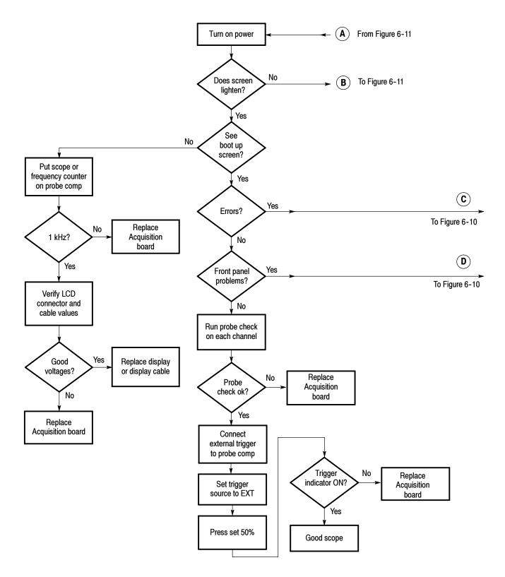
Figure 6-9: Oscilloscope troubleshooting tree (1 of 4)
