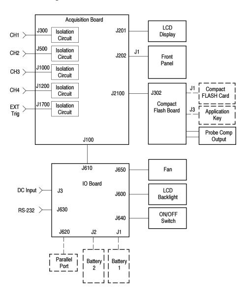
Figure 3-1: TPS2000 Series module-level block diagram, remove CH3 and CH4 for a 2-channel version
