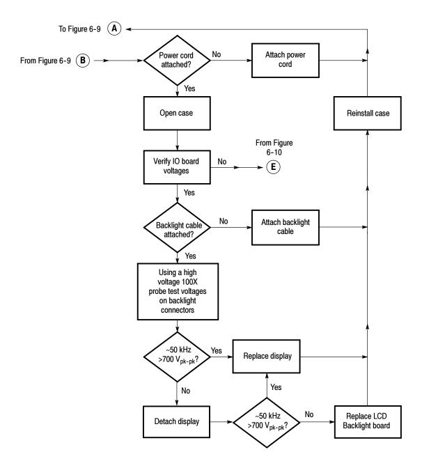
Figure 6-11: Oscilloscope troubleshooting tree (3 of 4)
