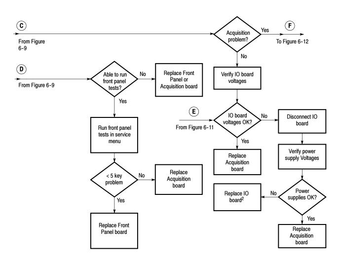
Figure 6-10: Oscilloscope troubleshooting tree (2 of 4)
