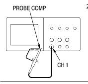
2. Set the switch to 10X on the P2200 probe and connect the probe to channel 1 on the oscilloscope . To do this, align the slot in the probe connector with the key on the CH1 BNC, push to connect, and twist to the right to lock the probe in place.
