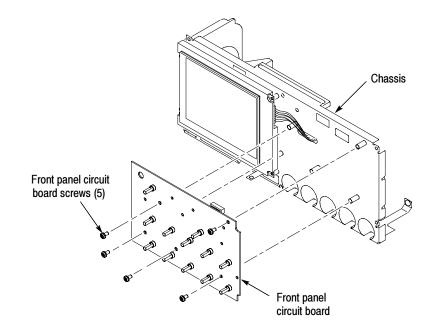
Figure 6-6: Removing the front-panel module
