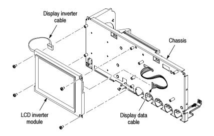
Figure 6-7: Removing the display module
