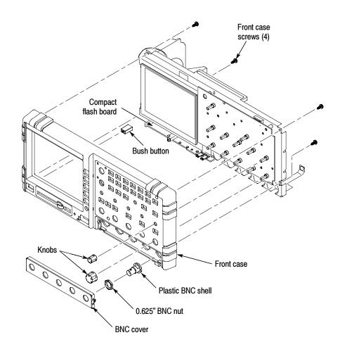
Figure 6-4: Removing the front case
