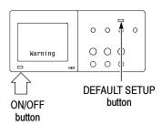
1. Power on the oscilloscope.
