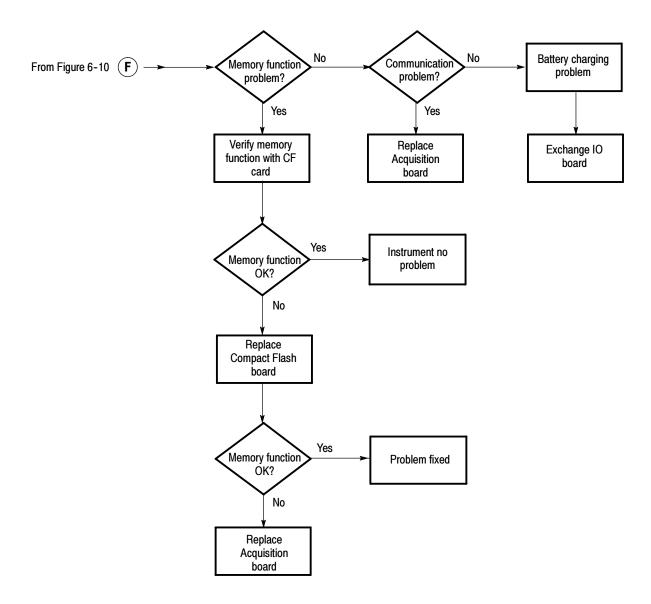
Figure 6-12: Oscilloscope troubleshooting tree (4 of 4)
