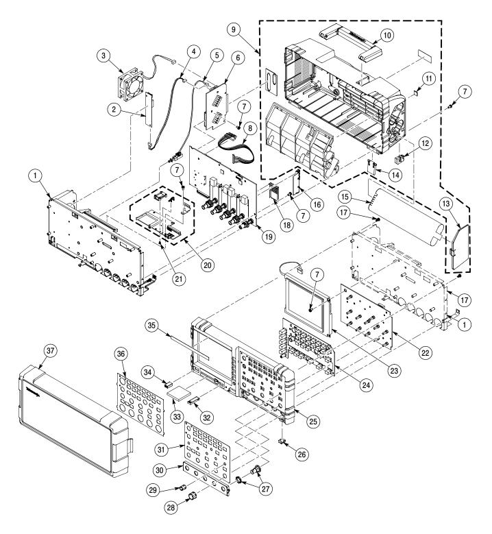
Figure 8-1: Exploded view diagram
