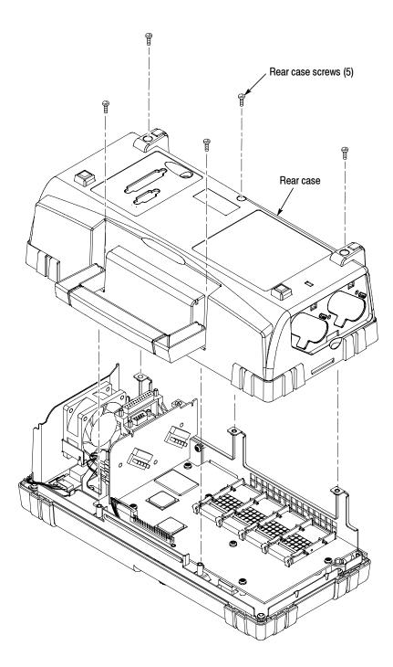
Figure 6-1: Removing and installing the rear case
